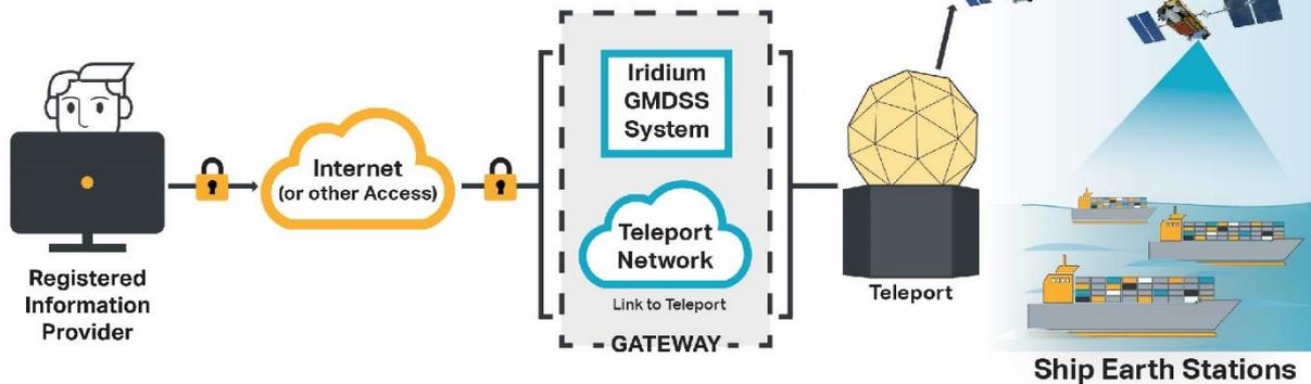
**Figure 2 – Basic concept of the Iridium SafetyCast service**
